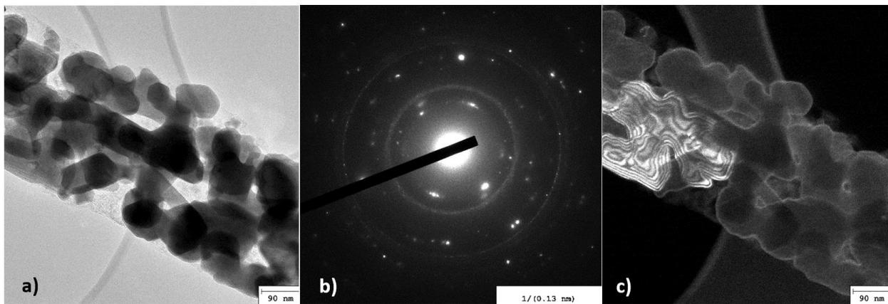
**Figure 2:** a) Bright-field TEM image of an 8YSZ nanofiber b) selected area electron diffraction pattern from the fiber c) Dark-field TEM image of the fiber.
