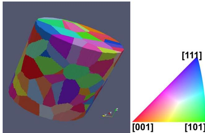
**Figure 1:** Simulated 3D-OMiTEM data of tessellated nano-structure after reconstruction in Dream3D. The colors indicate the grain orientation.
