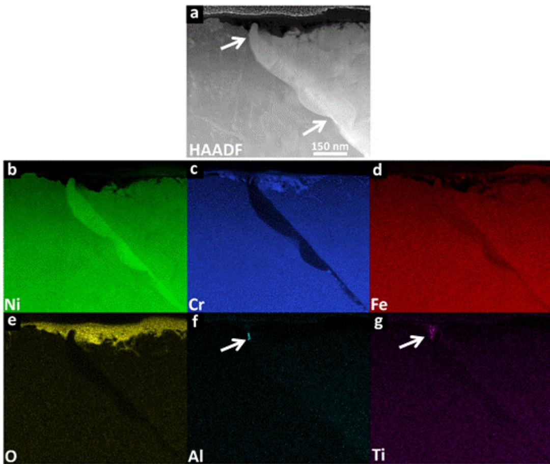
Figure 2: Detailed ATEM characterization of the R=1/24 (more oxidizing environmental exposure) sample. (a) STEM-HAADF image showing ~500 nm length (arrowed) of grain boundary which has migrated ~50 to ~100 nm in extent. (b)-(g) Elemental maps for (b) Ni, (c) Cr, (d) Fe, (e) O, (f) Al, and (g) Ti extracted from the STEM-EDX dataset showing the new migrated GB with the highly Cr-depleted region and the Al- and Ti- enrichment (arrowed).
