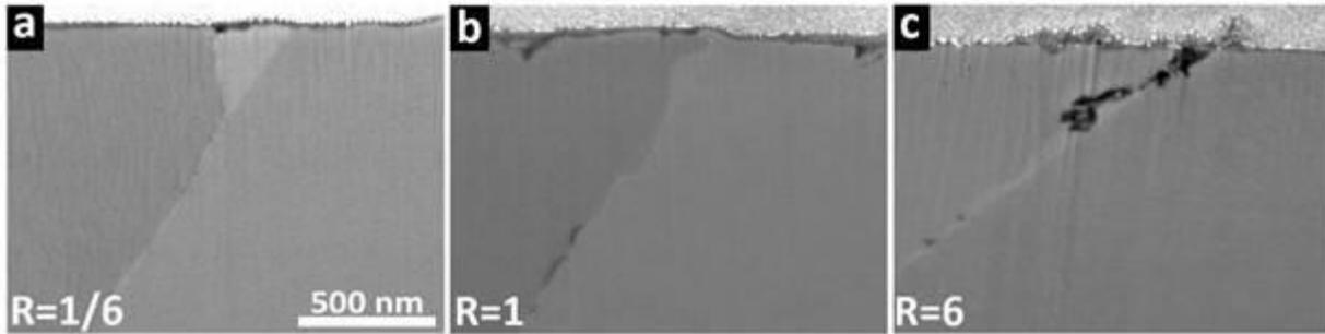
Figure 1: (a)-(c) SE images of FIB cross-section specimens prepared from samples exposed to H<sub>2</sub>-steam environments at 480 °C for 210 h for the different R values. For R<1, the environment is more oxidizing than the Ni/NiO transition whereas for R>1 the environment is more reducing.
