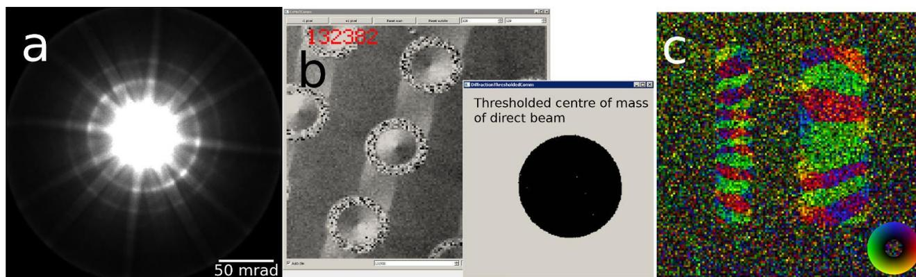
Fig. 1: a) STEM diffraction pattern of a perovskite oxide. b) Live DPC imaging of ferromagnetic domains using the `fpd_live_imaging` software package. c) DPC imaging of ferromagnetic domains using 1-bit detector depth, allowing for 80 us frame time.
