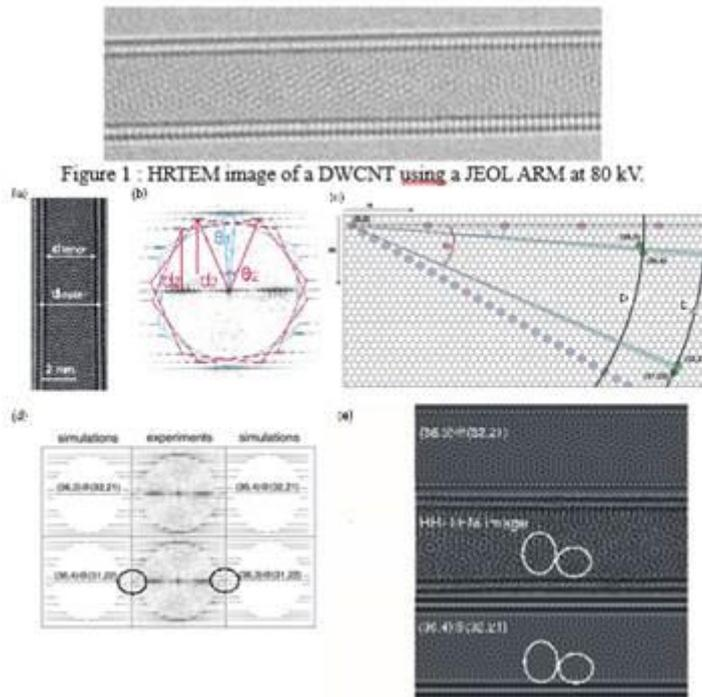
Figure 1 - HRTEM image of a DWCNT using a JEOL ARM at 80 kV.
