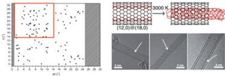
Figure 3 : Left: Statistical analysis plotting outer helicity versus helicity difference between outer and inner tubes: favored (red square) and non observed (dashed areas) configurations are marked . Right top : Relaxed configuration of forbidden DWNT after MC simulation. (c) Defected DWNTs observed experimentally where the inner tube diameters locally decrease (white arrows) as found in MC simulations.
