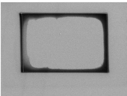
Fig. 1a: Inlens SE image of a contaminated area (width 5 $\mu\text{m}$ )
