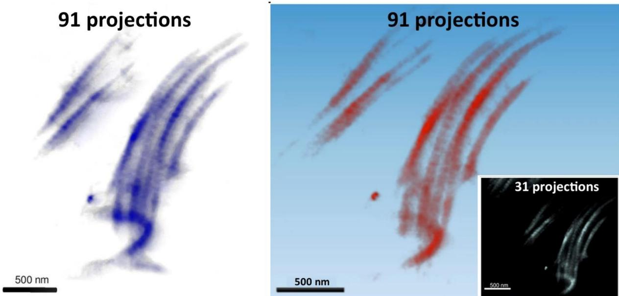
*Figure 2. Comparison between conventional Algebraic Iterative reconstruction (left) and CS-refined tomogram of the collagen sample. In both cases, 91 projections have been used for the reconstruction. Inset: CS-refined tomogram obtained with 31 projection images, where the fibrils are still clearly reconstructed. (Adapted from ref. [2]).*
