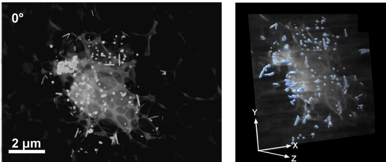
Figure 1. Left: DF T-SEM image of the graphene-ZnO hybrid structure obtained in at 0° tilt featuring mass-thickness contrast. Right: 3D reconstruction of the graphene-ZnO hybrid structure from the tilt series of T-SEM projections (light blue structures are ZnO nanostructures).
