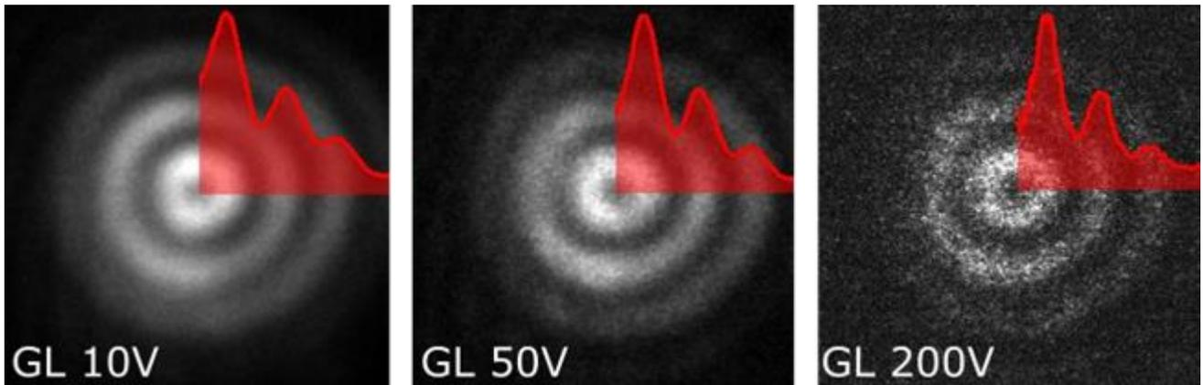
**Figure 1:** Images of the electron vortex beam for different gun lens excitations using a XFEG @ 200kV. An exposure time of 0.5 sec was used for all images. Insets show normalized and rotationally averaged intensity profiles.
