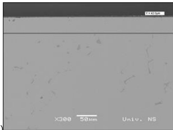
a) Fig. 2 - SEM microstructure of surface contamination: a) Directional growth of globules on grinding scratches; b) Contaminations globules
