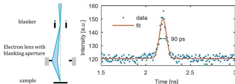
**Figure 3** The electron beam is pulsed using beam blanking technology, enabling a 90 ps pulse duration.
