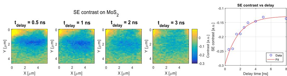
**Figure 4 Proof of principle pump probe measurements on MoS<sub>2</sub>. The laser induced SE yield images on the left indicate that laser excitation results in a reduction of the SE yield. An exponential fit shows a restoration time of  $1.8 \pm 1.1$  ns.**
