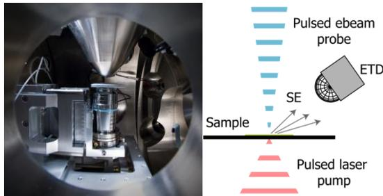
**Figure 2** The FEI Quanta 200 SEM based setup accommodates an inverted optical microscope underneath the sample, meaning that the specimen can be the subject of simultaneous electron and high NA optical imaging.
