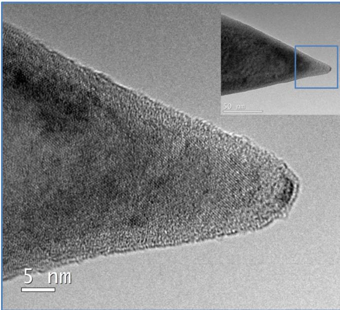
**Figure 2.** TEM image of the Si APT specimen following 900 eV argon ion milling shows significant reduction of the amorphous layer on the tip and sidewalls. The inset is a low magnification image with the area of interest marked.
