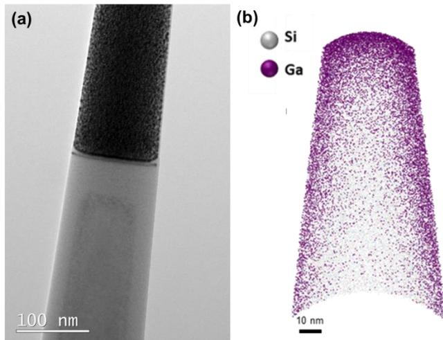
**Figure 1.** TEM image of a Si APT specimen as prepared **(a)** and Ga distribution from a three-dimensional APT reconstruction **(b)** after 30 keV FIB milling.
