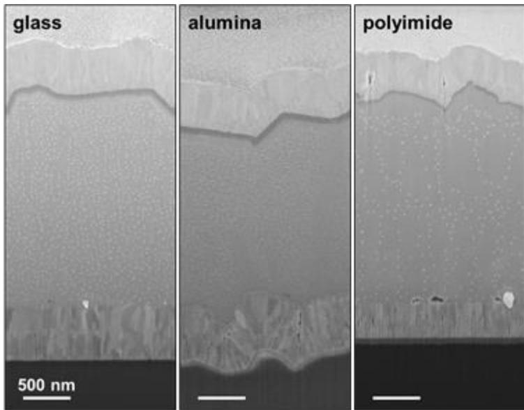
**Figure 1.** Cross sections of CIGS solar cells on glass, alumina and polyimide.
