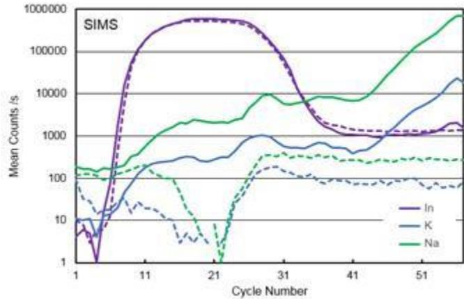
**Figure 2.** SIMS depth profiles for In, K, and Na for two CIGS solar cells with glass (solid lines) and alumina (dashed lines) substrates.
