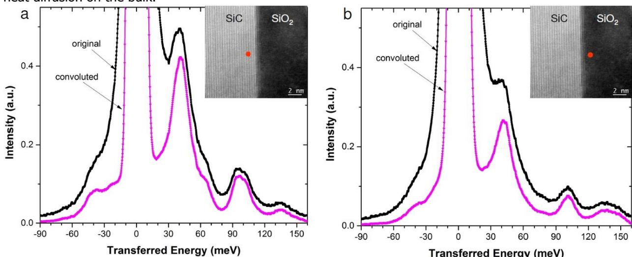
**Fig.1.** Vibrational spectroscopic spectra (black curves) acquired in both sides of the SiC/SiO<sub>2</sub> interface (inset). Note variations in the shape and amplitude of the resonances. Probe position is indicated by a red circle (~1 nm from the interface) in the inset. Deconvoluted spectra (magenta curve) using a Richardson-Lucy method [3] are also shown (3 iterations). We found the FWHM of the ZLP is reduced down to ~5 meV.
