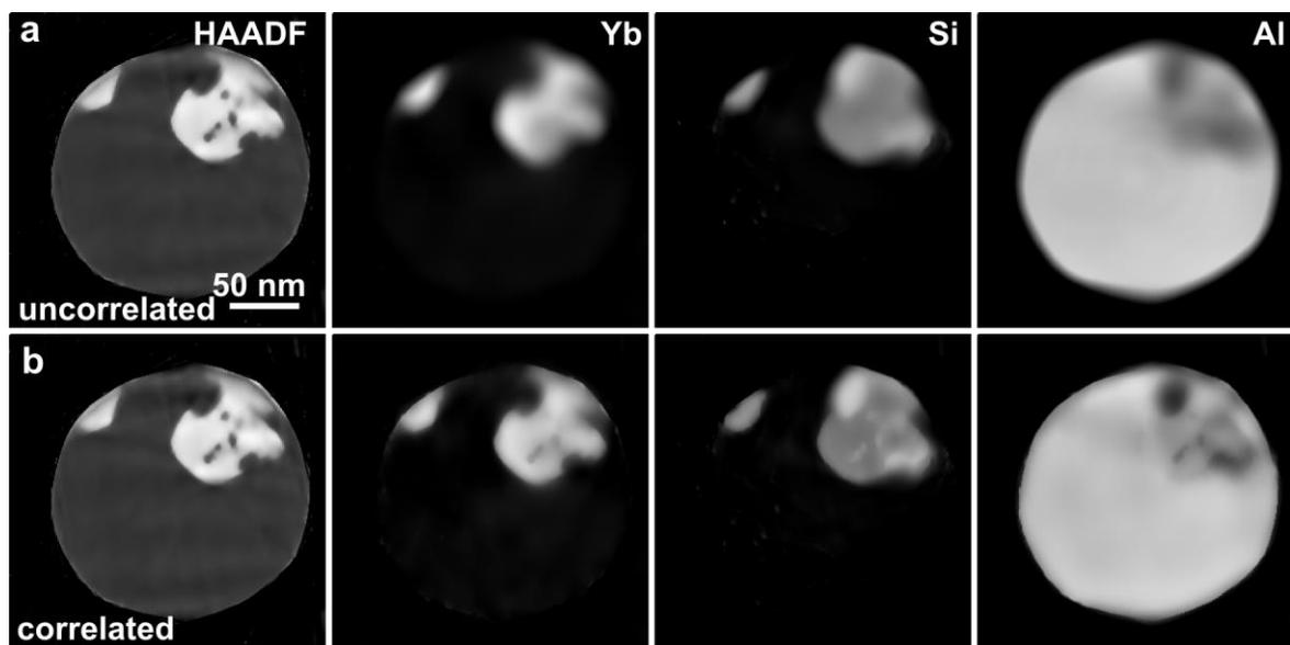
Fig. 2 Slice through (a) an uncorrelated and (b) a joint reconstruction of the HAADF STEM signal and EDXS elemental maps for Ytterbium, Silicon and Aluminum.
