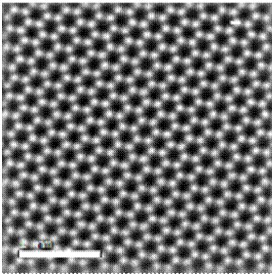
**Figure 1.** (left) The ptychographically reconstructed phase image of hBN. Unlike the simulation for neutral atoms, which shows a clear polarity between the N and B, the atoms show very similar phase in the experimental image.
