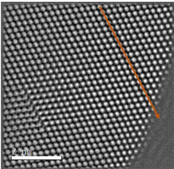
**Figure 2.** An experimental ptychographic phase image of a wedge sample of Pt recorded at 200 kV. Note the appearance of "donut"-like features in the thicker areas.
