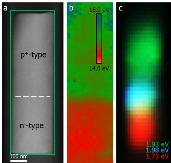
Fig. 3: (a) HAADF micrograph of a doped  $Ga_xIn_{(1-x)}P$  NW and corresponding (b) EELS bulk plasmon map and (c) CL map acquired in the green box showing how in both cases an energy shift from the n- to the p-segment occurs.
