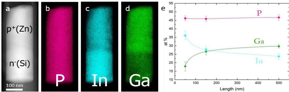
Fig. 2: (a) HAADF micrograph and corresponding EDX chemical maps showing the (b) phosphorous, (c) gallium and (d) indium content in doped  $Ga_xIn_{(1-x)}P$  NWs. (e) Compositional trend averaged on six different NWs at three different distances from the interface with the silicon at the bottom of the NW.
