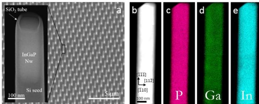
Fig. 1: (a) SEM image showing a region of InGaP NWs grown on Si(111). (b) HAADF and EDX maps of (c) phosphorous, (c) gallium and (d) indium content in undoped  $\text{Ga}_x\text{In}_{(1-x)}\text{P}$  NWs.
