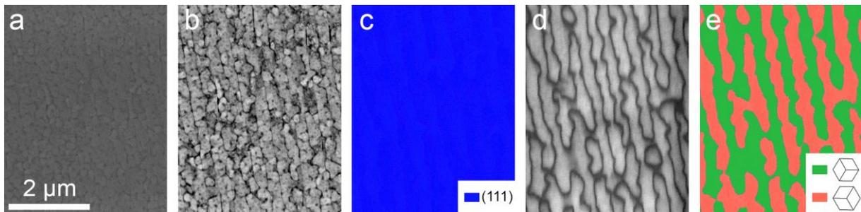
Figure 3: TiN electrode top view in a. secondary electron contrast, b. back scattered electron contrast, c. inverse pole figure (IPF) map of the (111) oriented TiN layer, d. image quality (IQ) map of (note boundary regions of quasi-symmetric grains with decreased quality factor), e. color coded map of the two possible orientations.
