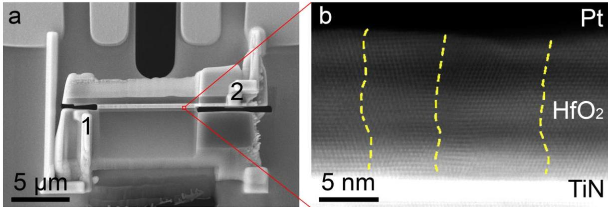
Figure 1: a. SEM image of a FIB prepared  $\text{HfO}_2$  device on a MEMS based chip used for in-situ biasing TEM experiments, contacts for electric field application are denoted as 1 (bottom TiN electrode) and 2 (top Pt electrode), b. corresponding high resolution HAADF-STEM image of the  $\text{HfO}_2$  layer and the corresponding electrode interfaces, boundaries between different orientation  $\text{HfO}_2$  grains are marked.
