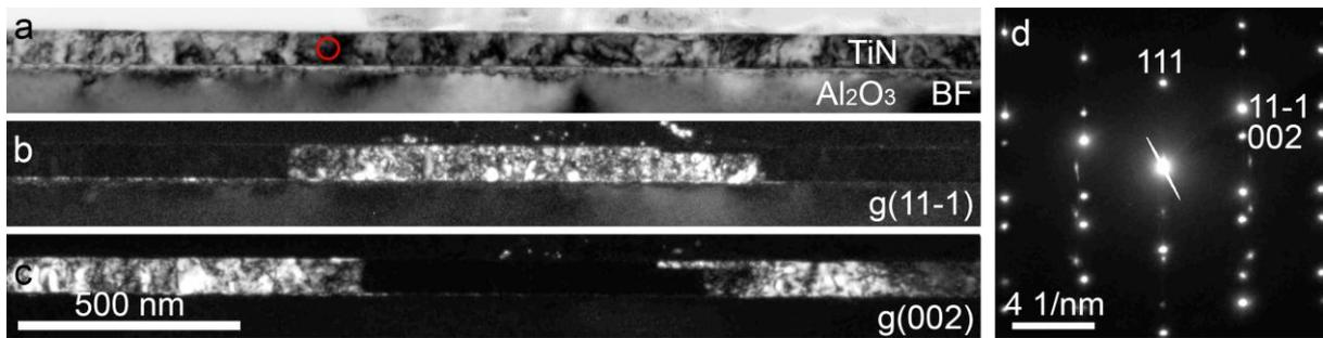
Figure 2: a. Bright-field cross sectional image of the TiN electrode/ $\text{Al}_2\text{O}_3$  interface region, b.  $g(11-1)$  dark-field image of the same region, c.  $g(002)$  dark-field image of the same region, d. corresponding NBD pattern, origin depicted in a.
