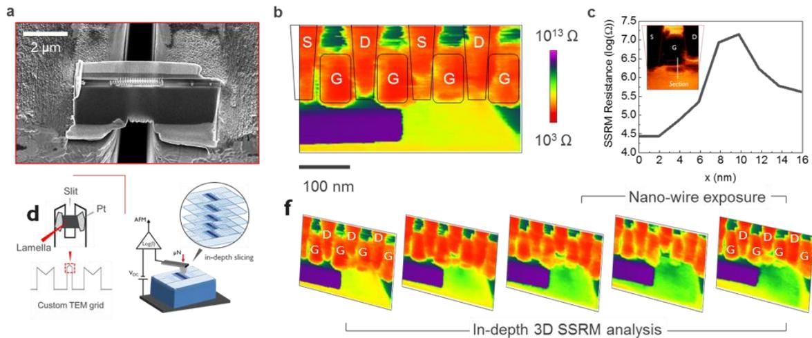
Figure 5 FIB-SEM image (a), first SSRM image (b), NW SSRM resistance profile (c), schematic of the SSRM set-up (d), in depth 3D SSRM sequence (f)
