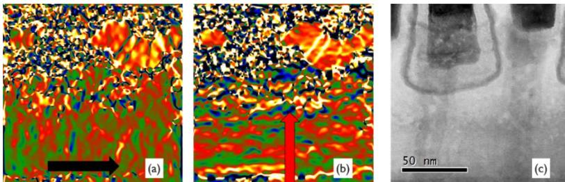
Figure 4 Strain analysis by GPA along (a) and perpendicular (b) to the NW, and correspondent ABF-STEM (c)
