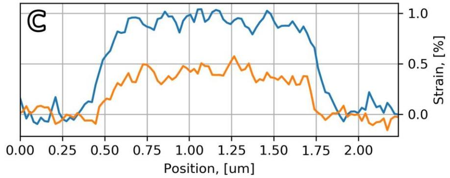
Fig. 1: a) STEM-DPC image showing the patterned ferromagnetic domains. b) Convergent beam diffraction pattern. Black arrow: direct beam, used to extract magnetic information. White arrow: diffraction spots, used to find structural information. c) Strain in the 3<sup>rd</sup> stripe from the left, in the long axis direction (orange) and the short axis direction (blue).
