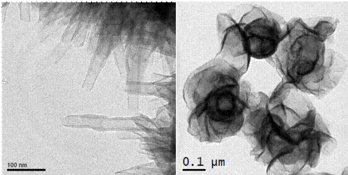
Figure: Transmission Electron Micrographs of (a)MoO<sub>(3-x)</sub> nanotubes and (b)MoS<sub>2</sub> nanosheets
