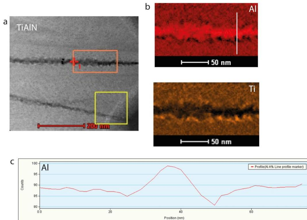
Figure 1. (a) HAADF STEM image of TiAlN grain boundary and surrounding TiAlN grains. (b) Ti and Al EDX maps of TiAlN grain boundary seen in (a). (c) Line profile, top - bottom, showing the variation of Al over TiAlN grain boundary.
