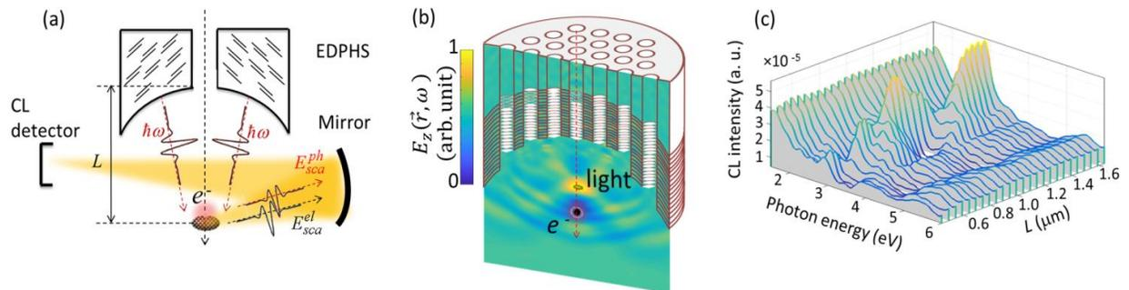
Fig. 1. (a) an electron interacting with the EDPHS and the sample. (b) Interaction of the electron with a precisely engineered EDPHS will result in a focused and coherent transition radiation. The emitted light which is detected then by a CL setup will demonstrate interferences within the energy-distance map.
