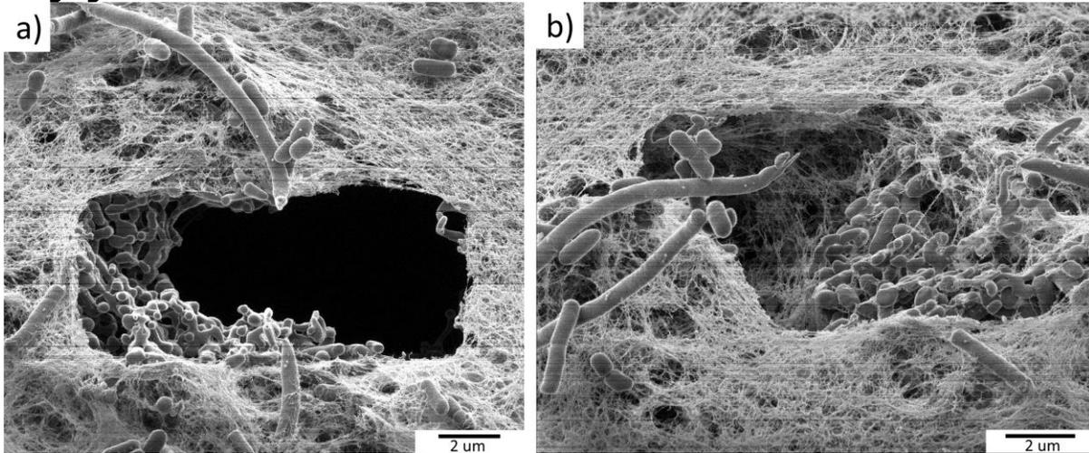
**Figure 3: a) A slot milled to the agar substrate from an 45 angle with neon and imaged from 90 degree angle. b) The same milled area imaged with a 45 tilt and a 90 rotation.**
