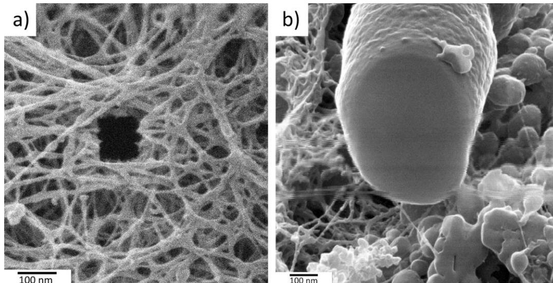
**Figure 2: a) 100 x 100 nm area milled to the agar substrate b) He-milled bacteria showing up cut-off surface and a half-away cut phage particle on top of it. Milling was done from the 45 angle and imaging after 180 rotation.**
