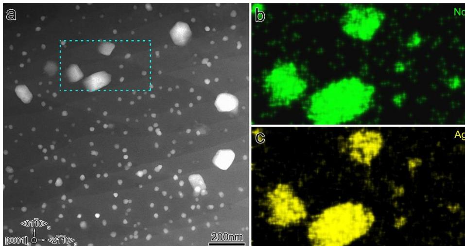
Figure 2. (a) HAADF-STEM image showing the equilibrium precipitate phase and (b, c) STEM-EDS maps of the equilibrium phase particles outlined in the blue frame in (a): (b) Nd map, (c) Ag map.
