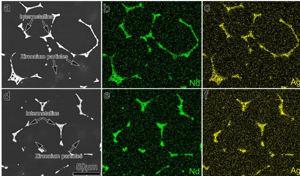
Figure 1. BSE images showing equilibrium intermetallic phase in (a) as-cast, and (b) solution treated samples. (c-f) SEM-EDS mapping analysis of the equilibrium intermetallic phase: (b, e) Nd maps, (c, f) Ag maps.
