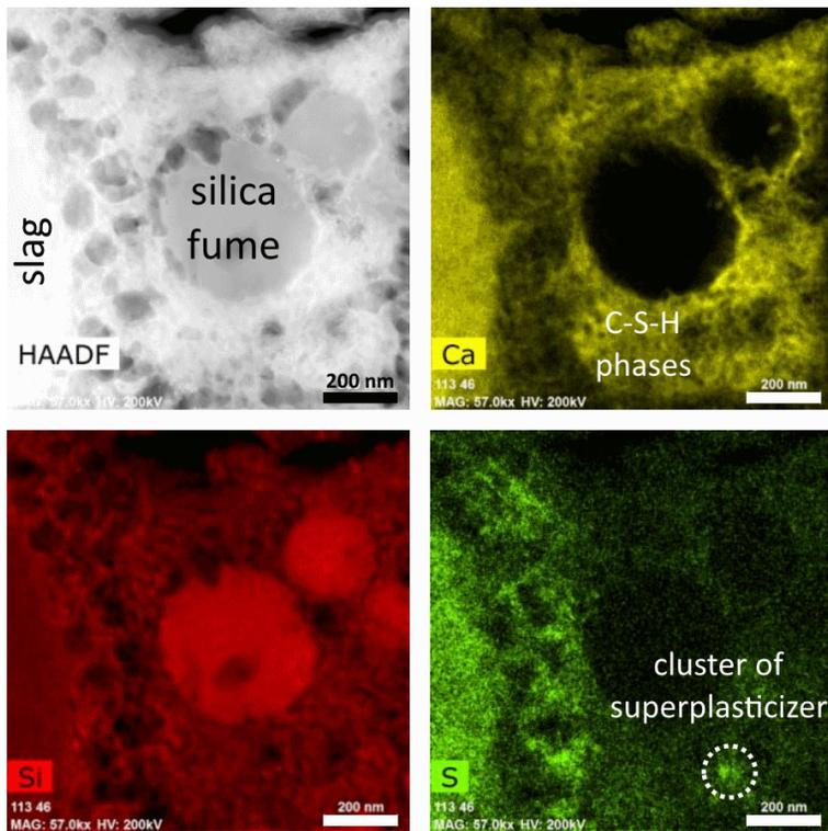
**Fig. 2:** HAADF-STEM image and EDS elemental distribution maps revealing a cluster of superplasticizer molecules in the cement paste matrix.
