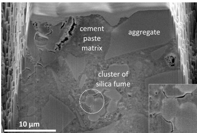
**Fig. 1:** SEM SE image from "Slice & View" tomography showing minute cracks close to a cluster of silica fume particles.
