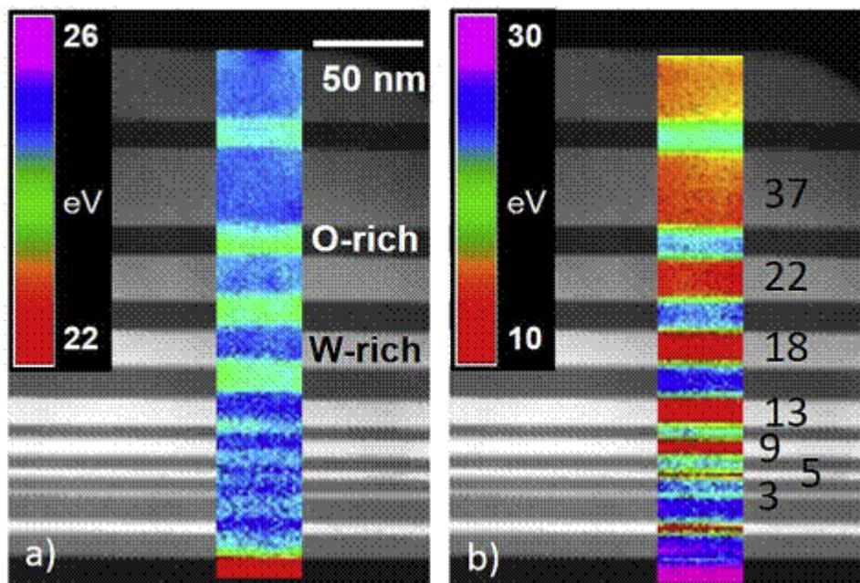
Figure 1: Color-maps of a) center and b) FWHM extracted after NLLS fitting with a Gaussian curve, of the most intense low-loss peak, superposed on the original dark-field STEM image from a sample with various metallic and oxide thicknesses.
