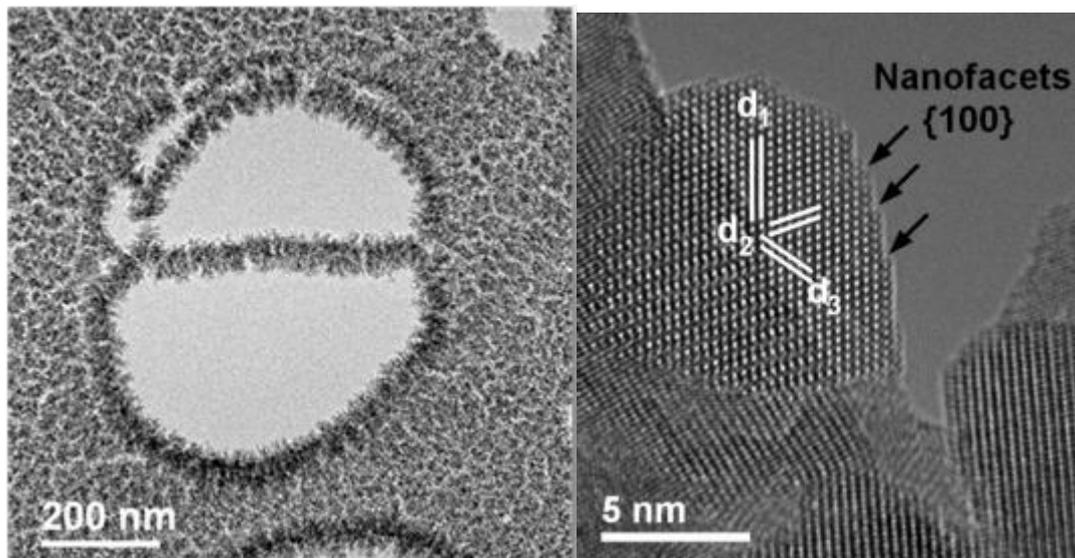
Figure 1: Platinum doped cerium oxide deposited on TEM membrane grid. HRTEM image of the surface layer: the crystallized grain is identified as CeO<sub>2</sub> and exhibits {100} type nanofacets.
