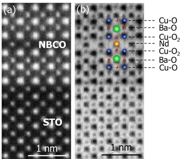
Figure 1: (a) HAADF- and (b) ABF-STEM images of the NBCO/STO interface with an overlay of the NBCO structural model.
