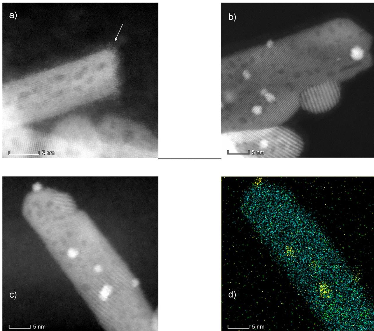
Figure 1 - CeO<sub>x</sub> porous nanorods appear highly crystalline in the HAADF-STEM image (a), before the deposition of Au NPs, with a thin layer of disordered ZnO (indicated by the arrow) covering the nanorods. Very small Au NPs (b) anchored on the porous CeO<sub>x</sub>/ZnO nanorods. HAADF-STEM image (c) and corresponding EDS-SI map (d) of the resulting catalyst material showing the distribution of Au (yellow), Ce (blue) and Zn (green).
