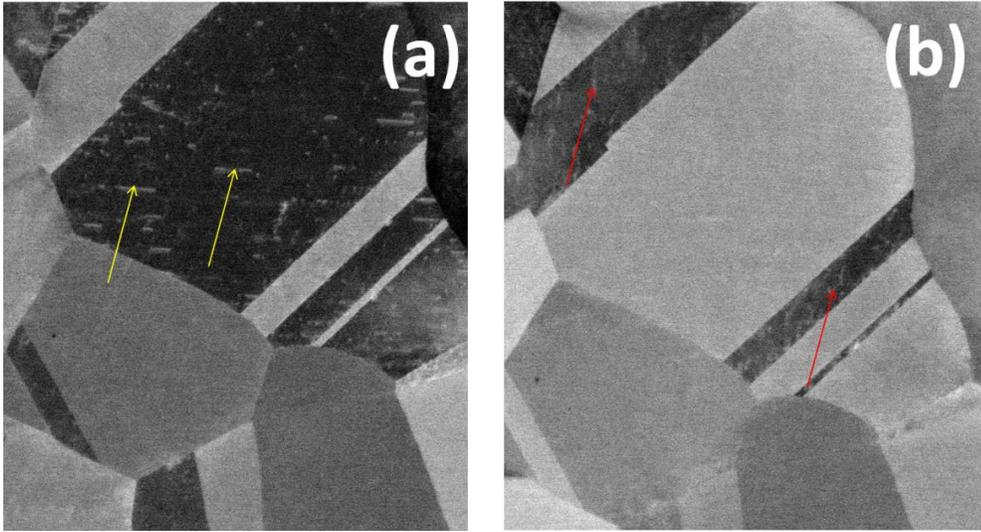
**Figure 1: Images extracted from a rotational series, where the dislocations (red arrow) and stacking faults (yellow arrow) can be seen in several grains for particular orientations.**
