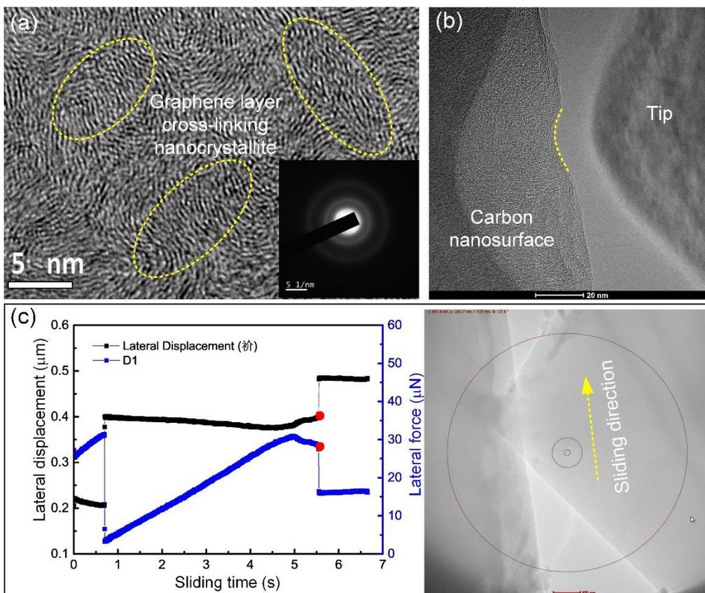
Figure 1 (a) The high resolution TEM image of the carbon nanosurface from plan view, graphene layer cross-linking nanocrystallites can be found in the nanosurface; (b) The TEM image of carbon nanosurface and tip
