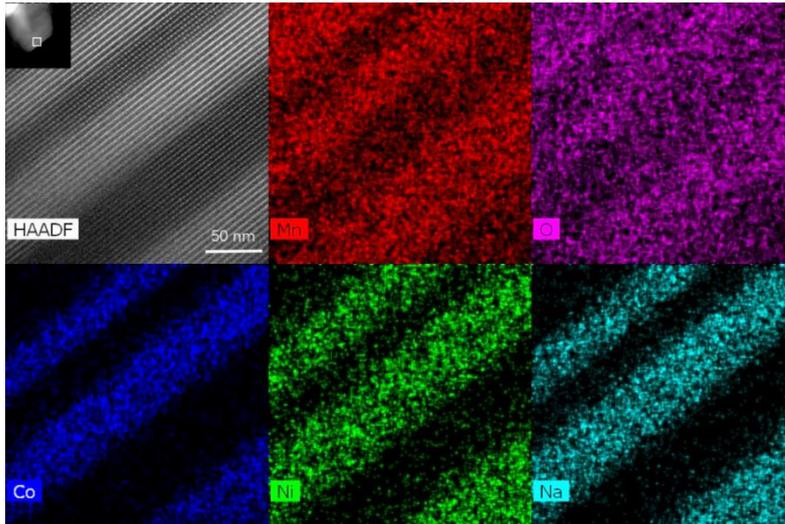
Fig 2 the epitaxial structure and elemental segregation of P3-O3' layered oxides
