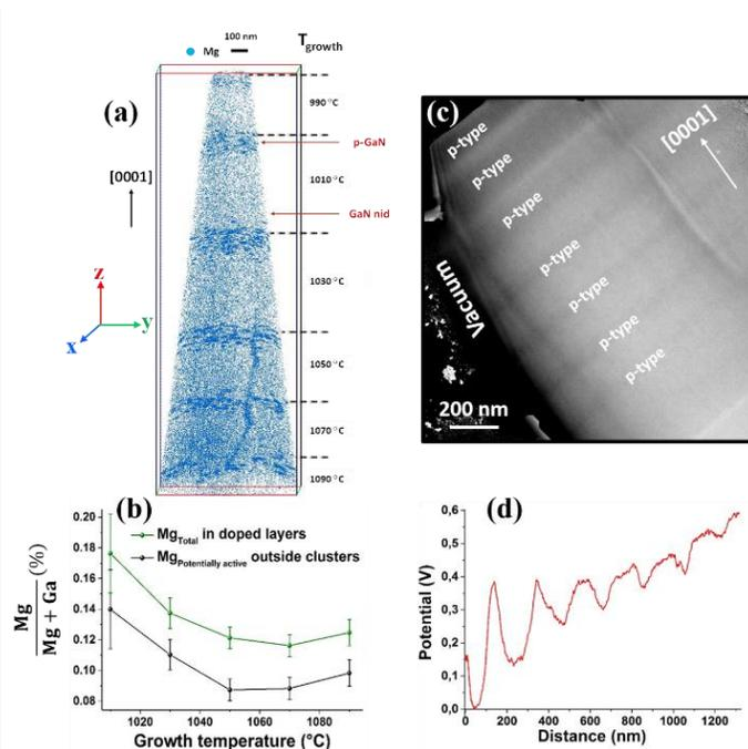
Figure 2: (a) APT 3D reconstruction of detected Mg atoms in blue (b) Global concentration of Mg in doped layers in green and Mg concentration outside clusters and threading dislocation in black (c) Potential map including all the layers acquired at 400 °C in-situ heating temperature to increase the number of measured carriers (d) Potential profile across all the series of doped and undoped layers.
