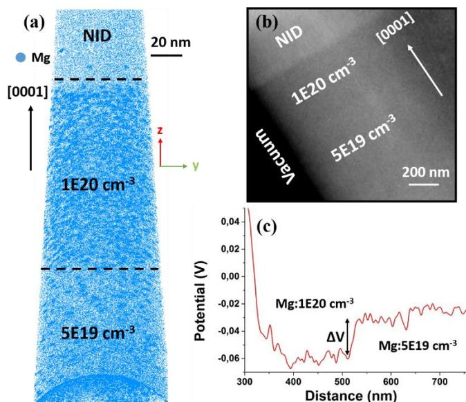
Figure 1: (a) 2D projection of Mg atoms detected by APT in blue (b) Potential map of the sample acquired at an in-situ heating temperature of 400 °C. (c) Potential profile across the two GaN doped layers at  $1E20\text{ cm}^{-3}$  and  $5E19\text{ cm}^{-3}$ .
