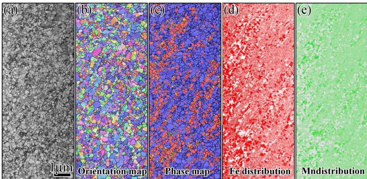
Fig.1 (a) TKD pattern quality map of the TWIP steel after 12-revolutions HPT; (b) TKD orientation map; (c) TKD phase map with austenite in blue, ferrite in red and M<sub>23</sub>C<sub>6</sub> carbide in yellow; (d) and (e) EDS element maps showing Fe and Mn K $\alpha$  X-ray counts, respectively.
