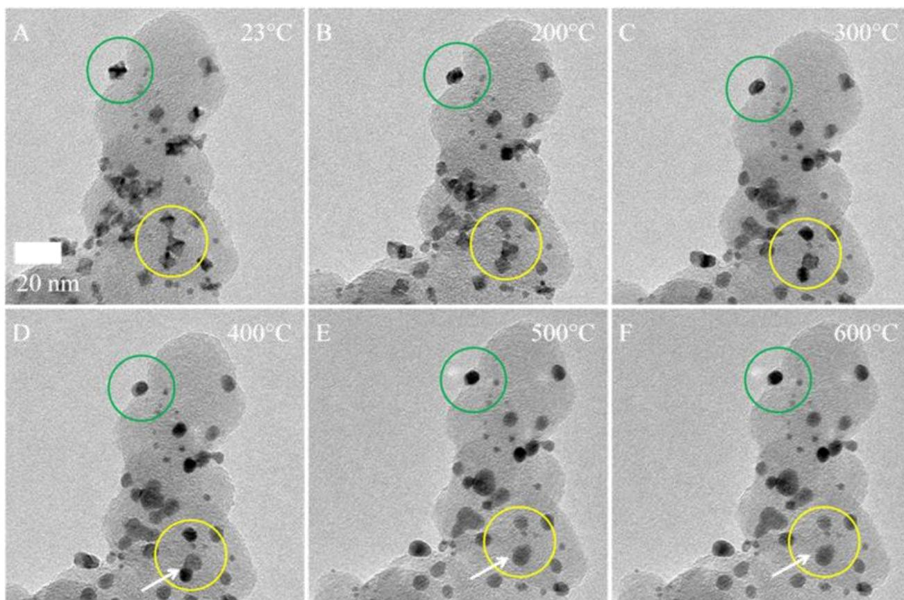
**Figure 1.** (A-F) TEM image series of PtNi<sub>1.5</sub> octahedral NPs under in situ thermal heating conditions from 23 °C to 600 °C. Green and yellow circles mark identical NPs at different temperatures. The arrows indicate coalescence of neighboring particles.
