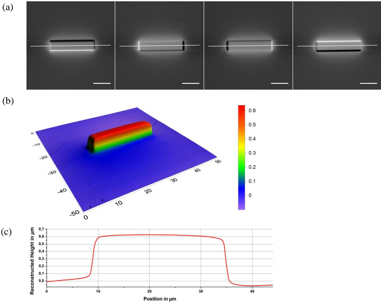
**Figure 1:** 4Q BSE images with 10  $\mu\text{m}$  scale bar (a), height map with scale in  $\mu\text{m}$  (b) and extracted line profile (c) of deposited Pt structure
