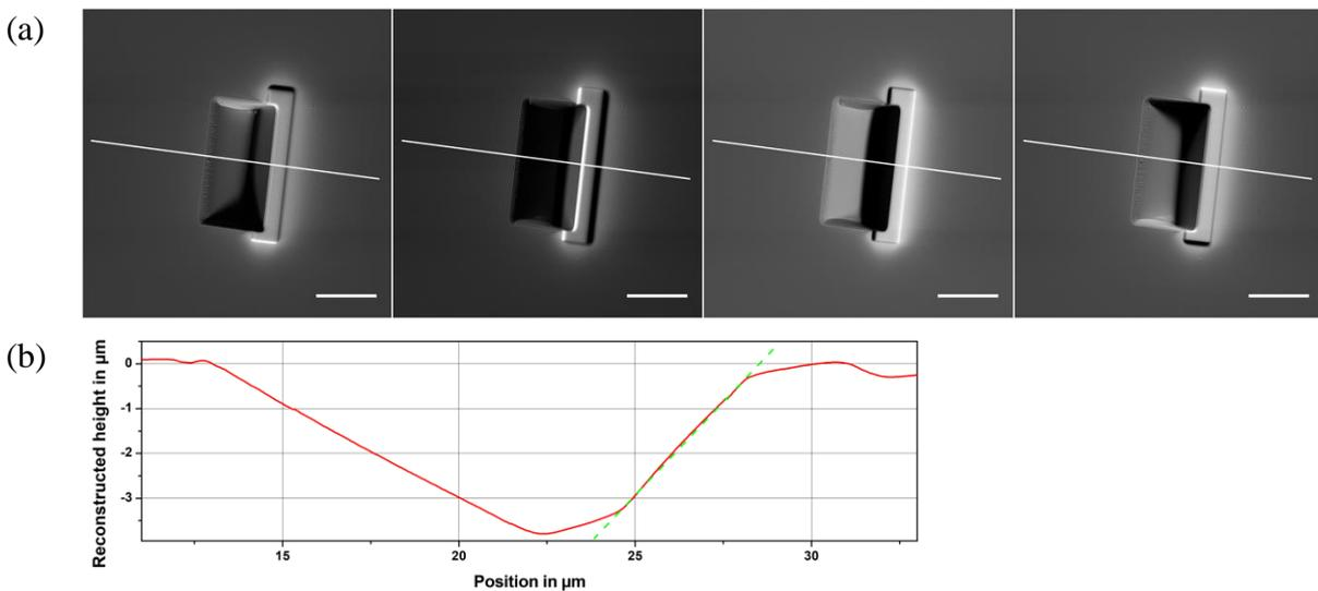
**Figure 2:** 4Q BSE images with 10  $\mu\text{m}$  scale bar (a) and line profile (b) across milled Si structure, note that the cross section surface is not vertical since the specimen is tilted by  $15^\circ$  during 4Q-imaging
