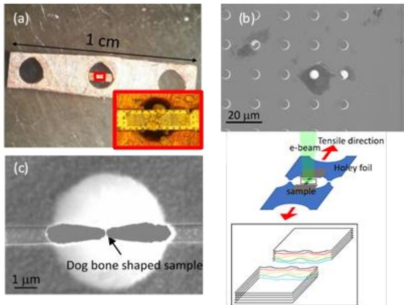
Figure 2 (a) A homemade sample stage to perform tensile test for two dimensional nanomaterials in TEM. Inset: thin foil attached on a smaller copper bridge. (b) A flake of sample indicated by an arrow covers a hole on the thin foil. (c) A dog-bone shaped sample prepared by FIB. (d) Schematic of a tensile experiment process in TEM.
