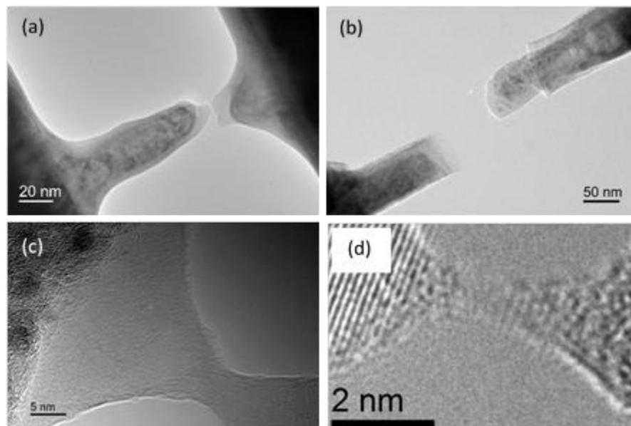
Figure 2 (a) and (b) A sample after being pulled to fracture using this sample stage. (c) and (d) A deformation process at high magnification observed during the ductile mode.
