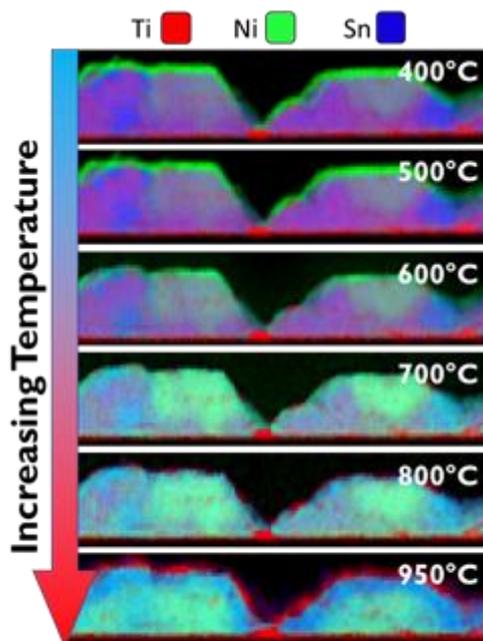
*Elemental false-colour visualisation taken from STEM-EELS annealing series of a phase segregated TiNiSn thin film.*
