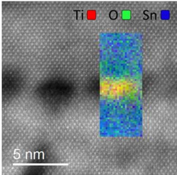
*Column Resolved STEM-HAADF image of TiO nano-inclusions in TiNiSn thin film. Overlay is false colour elemental map from STEM-EELS spectrum image analysis.*
