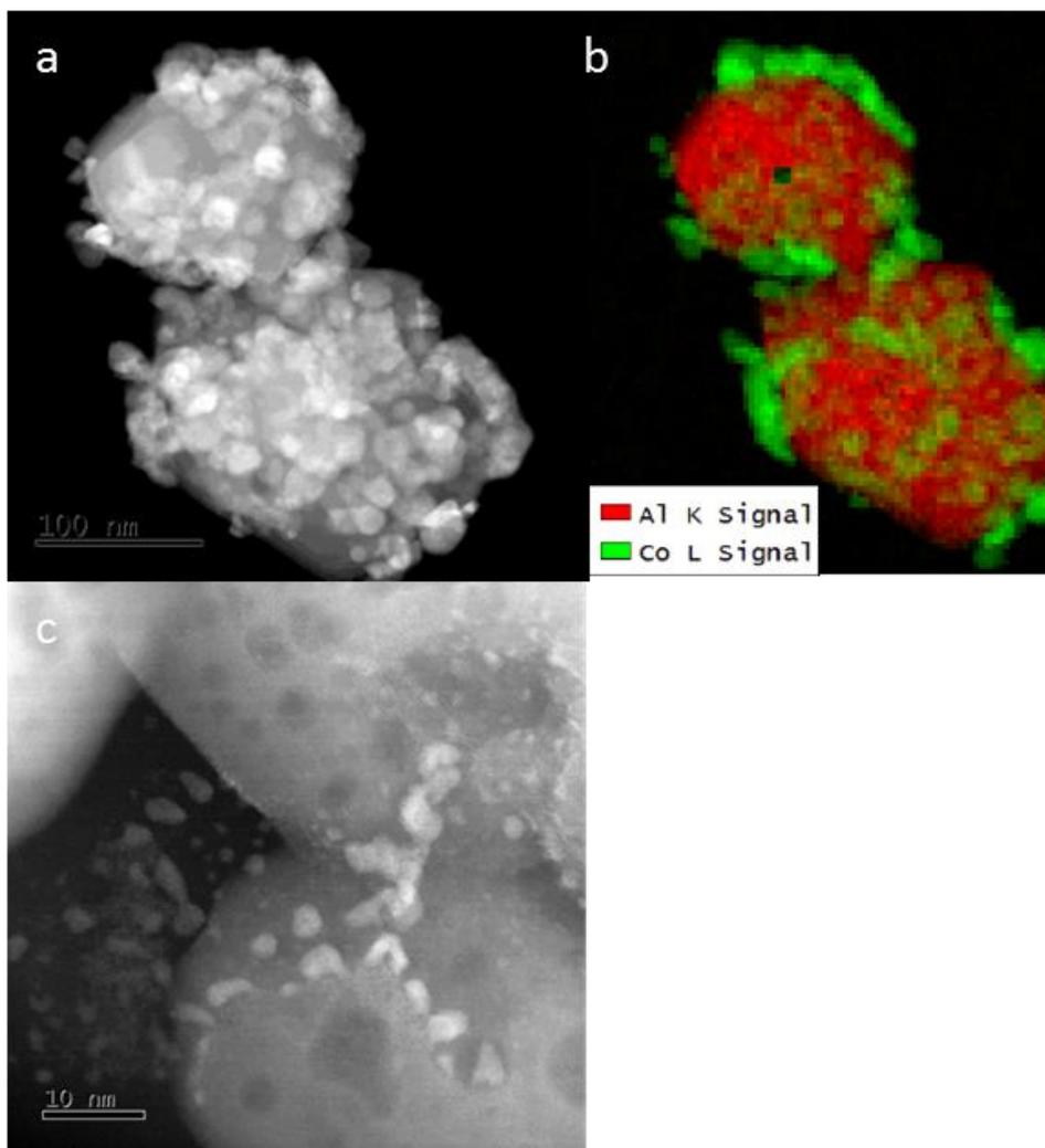
Figure 2: HAADF STEM image (a), STEM Al and Co EDX map (b) of Co/ $\alpha$ -Al<sub>2</sub>O<sub>3</sub> RO treated sample; HAADF STEM image (c) of Pt doped Co/ $\alpha$ -Al<sub>2</sub>O<sub>3</sub>.
