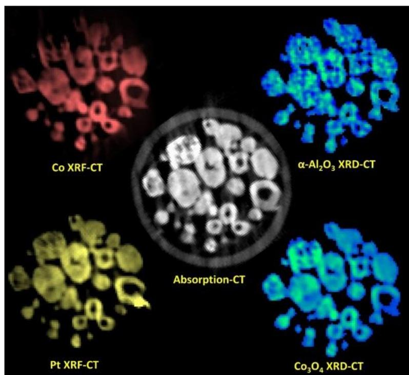
Figure 1: Absorption-CT, Co and Pt XRF-CT and XRD-CT reconstructions of  $\text{Al}_2\text{O}_3$  and  $\text{Co}_3\text{O}_4$  area (parent material) acquired at I18
