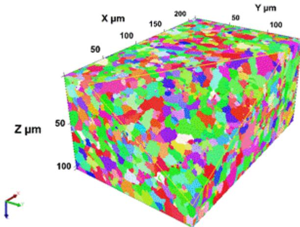
Figure 2. 3D reconstruction of EBSD x IPF data acquired using automated SSBIB tomography. The volume is  $213 \times 141 \times 103 \text{ } \mu\text{m}^3$  with  $0.5 \times 0.5 \times 0.7 \text{ } \mu\text{m}^3$  voxels. Milling used 8 keV Argon ions at  $5^\circ$  incidence for 7 minutes per slice, followed by EBSD acquisition of 20 minutes per slice.
