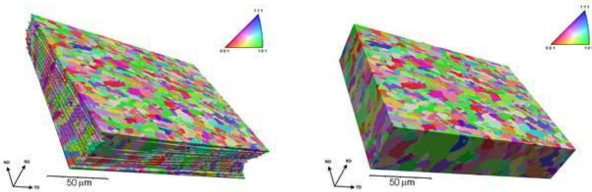
Figure 1. Left: 3D volume reconstructed from aligning 40 consecutive mechanically polished slices of a dual-phase steel. Right: Cropped to the volume common in all slices ( $185 \times 135 \times 40 \text{ } \mu\text{m}^3$ ), losing 17% of the data.
