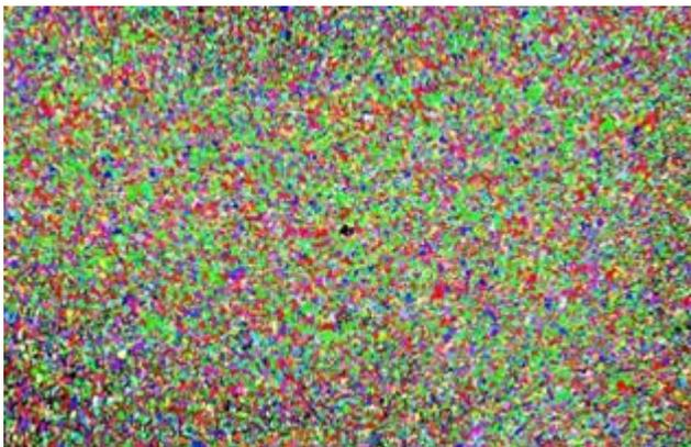
Figure 3. BIB produces polished surfaces much larger than  $1 \text{ mm}^2$ . A  $2.0 \times 1.3 \text{ mm}^2$  EBSD x IPF map of the top surface of the same sample is shown. The pixel size is  $0.54 \times 0.54 \text{ } \mu\text{m}^2$ . The edges of sample areas this large are difficult to keep in perfect focus, which results in an increase in unindexed (dark) pixels.
