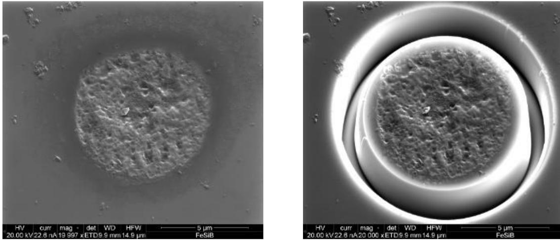
FIGURE 1. SEM images obtained during FIB SEM residual stresses measurement in the subsurface volumes of the  $\text{Fe}_{80}\text{Si}_{11}\text{B}_9$  sample. Different approaches were used to evaluate the strain relaxation.
