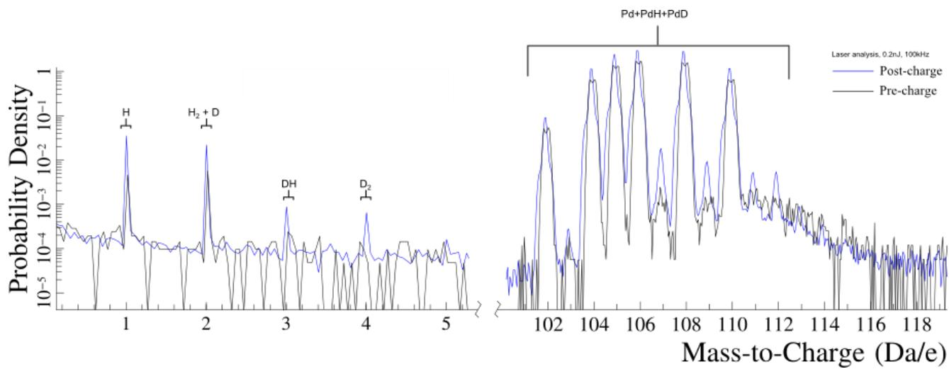
Figure 1: APT mass spectrum showing uptake of Deuterium in a Pd Alloy, with in-situ D charging (1 atm abs).
