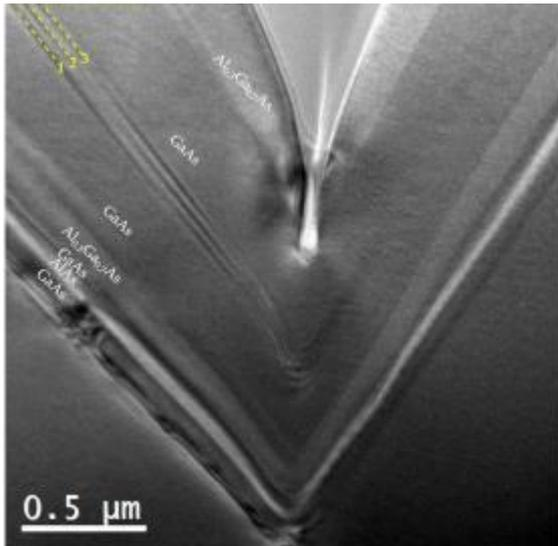
**Figure 1:** Transmission electron microscopy (TEM) cross-sectional overview of a triple pyramidal QD system. The position of the InGaAs (QD) layers is marked by 1, 2 & 3.
