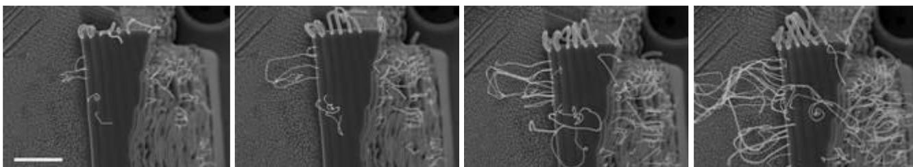
**Figure 3.** Nanowires growing from Pt-Ga substrate (platinum deposited by Ga FIB) at 700°C in pure hydrogen environment (H<sub>2</sub> pressure: 50 Pa). Average time interval between images: 1.5 minute. Scale bar: 4 μm.
