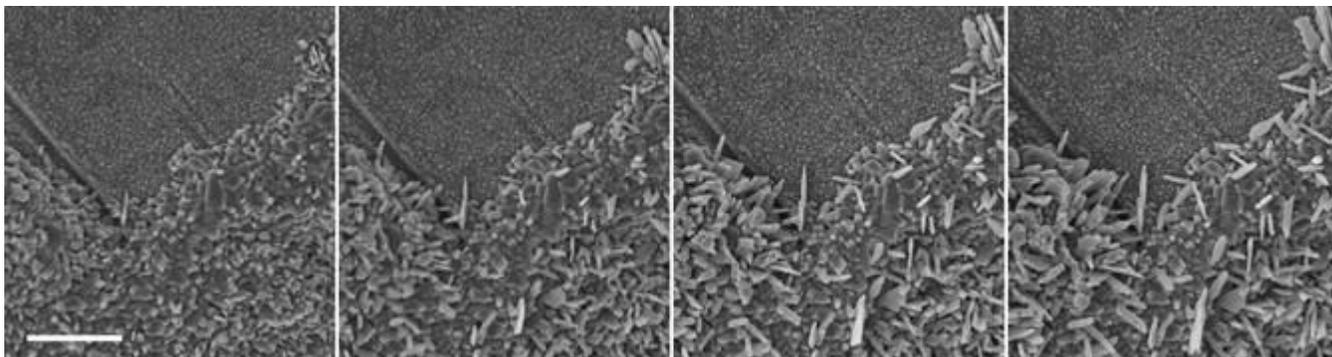
**Figure 2.** Evolution of rutile (TiO<sub>2</sub>) nanowires in acetone vapor (100 Pa) on Ti substrate heated to 850°C in FIB-SEM reactor. Time step between images: 4 minutes. Scale bar: 2 μm.
