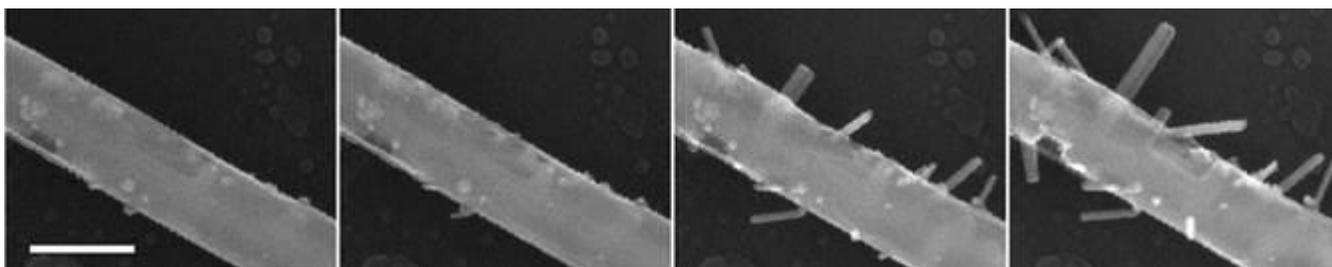
**Figure 4.** An image sequence (6 minutes duration) of tungsten oxide nanowires growth from tungsten disulfide nanotube during oxidation reaction (725°C, H<sub>2</sub>O vapor in reactor). Scale bar: 100 nm.
