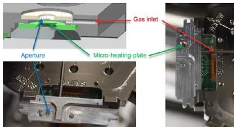
**Figure 1.** FIB-SEM reactor connected to multi-sample holder of a Helios G4 UX system, which controls heating of the micro-heating-plate (up to 1200°C). Pressure limiting aperture separates overpressure in the reactor (up to 100 Pa) from vacuum environment ( $<10^{-2}$  Pa) in SEM chamber.
