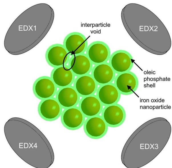
Fig. 2: FCC packed iron oxide nanoparticles with oleic phosphate shell in viewing direction [110]. Sample and detector layout corresponds to acquisition parameters of Fig. 3
