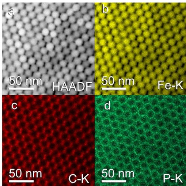
Fig. 3: HAADF and spectrum image of iron oxide - oleic phosphate nanocomposite. All four EDS detectors used.
