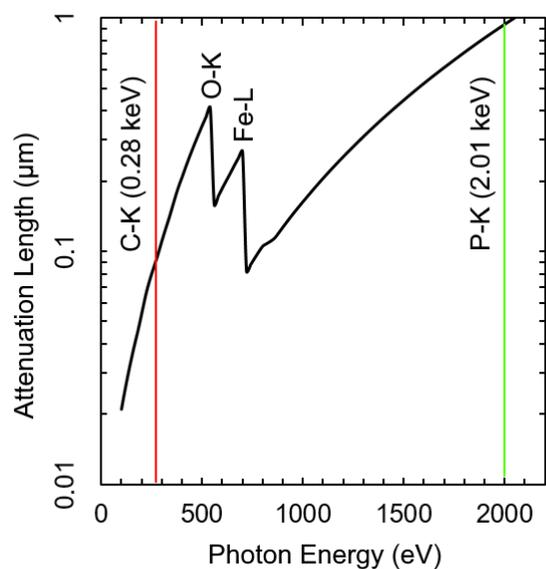
Fig. 1: Calculated attenuation length of x-rays in  $\text{Fe}_3\text{O}_4$ .
