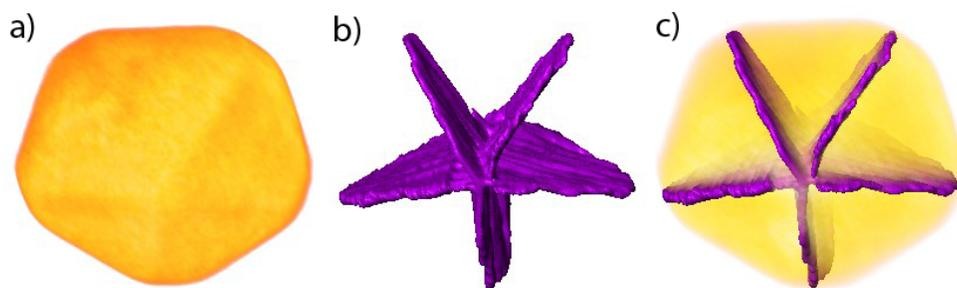
**Figure 1.** 3D visualization of (a) The HAADF-STEM reconstruction (b) The twin planes segmented from the LAADF-STEM reconstruction (c) Both volumes are superimposed.
