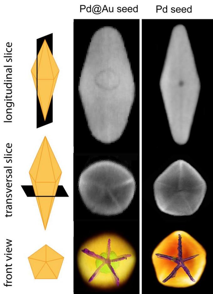
**Figure 2.** Top row: Longitudinal orthoslices through the HAADF-STEM reconstruction of bipyramids from Pd@Au and Pd seed. Middle row: Transversal orthoslices through the LAADF-STEM reconstruction, from which the twins can be segmented. Bottom row: Superposition of the segmented seed and twin planes.
