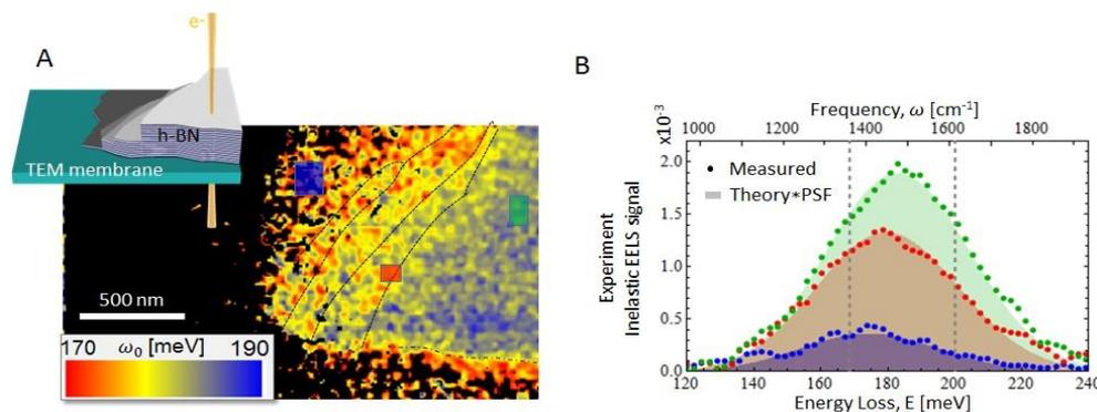
**Figure:** A) Peak position EELS map of a hBN flake (sample geometry is displayed in the inset showing the variation of thickness from a few monolayers to 30 nm). B) Experimental EELS spectra
