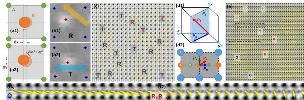
FIG. 1. (a1,a2) and (d1,d2) structural models; (b1,b2) and (c) HAADF and ABF images of KNN-based material with polarization map, R+T; (e) ABF image of BT-based material with polarization map, R+T+O; (f1,f2) Gradual polarization rotation between R, O, and T.
