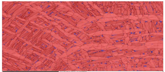
Figure 1b. Example phase map of a 2 phase Ti64 alloy collected using a CMOS based detector at 1000 pps. Red - alpha Ti, Blue - beta Ti. Raw data (approximately 99% indexing). Scale bar marks 50 um. Sample courtesy of Materials Consult, UK.
