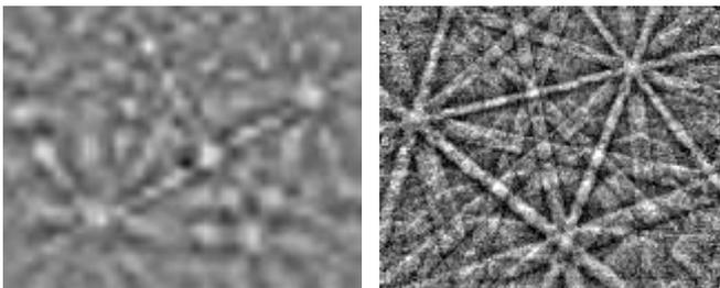
Figure 1a. EBSPs from Ni. Left - CCD based detector collected at 1500 pps. Right - CMOS based detector collected at 3000 pps.
