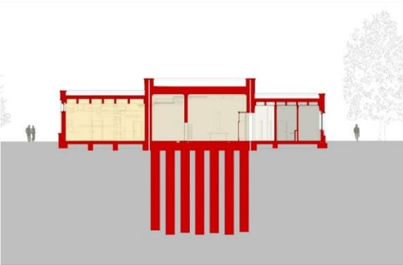
Fig. 3: Grounding of the building on 122 piles (courtesy of Noefer Architekten)
